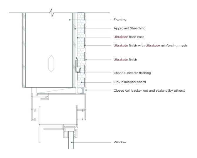
NOTE 1: Ensure the diverter flashing extends 6 inches beyond opening on either side of the opening to allow potential moisture to drain down the wall to the side of the opening. Maintain a minimum of 1/4" EPS insulation thickness, ensure the diverter flashing has positive slope to provide a means for drainage.
